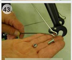
Anchor wires attach with screws into the holes in the rear fork
