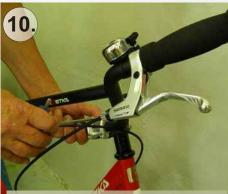
The handlebars is necessary strongly to fixed by tools to the higher position
