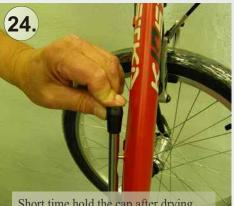
Short time hold the cap after drying the glue is attached to stand 111.12
