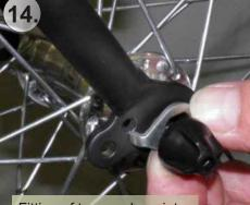
Fitting of two washers into the holes on the fork
