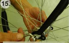
The quick charge from the left side mounted the wheels and properly tightened. When attaching the wheels to make sure that the wheel rotation direction marked on the tires
