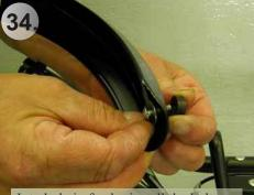
Into hole in fender install the bolt with washer and through the plastic screwed to the body surface
