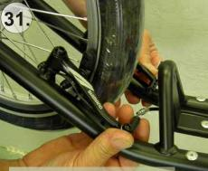
Extend brake shoes and remove the wheel from the fork
