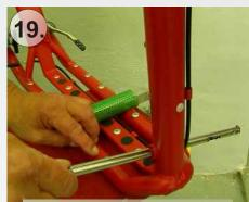
Metal tube of the stand setting up and installation of direction from the upper level on the top position
