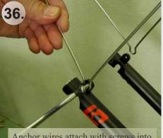
Anchor wires attach with screws into the holes in the rear fork
