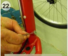
Put the screw into slot hole and properly tighten by tools
